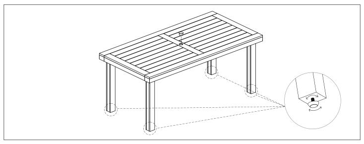
Using a second person to assist you, turn assembly upright. Assembly is now complete and the product is ready for use. Adjustable levelers are located on the bottom of each leg and may be adjusted by turning outwards, counter-clockwise to help account for uneven surfaces. NOTE: Hardware may loosen over time. Periodically check that all connections remain tight and adjust as needed. Insert Parasol Cap (C).
