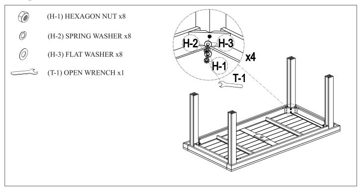
Place Table Top Panel (A) upside down on a padded non - marring surface. Insert bolts on Leg (B) through predrilled holes in corners of apron. Secure bolts with Flat Washers (H-3), Spring Washers (H-2) and Hexagon Nuts (H-1), stacking the hardware in the order as shown. Loosely install hardware on all bolts. Fully tighten using Open Wrench (T-1) after all hardware is installed. DO NOT OVER TIGHTEN. Repeat for remaining Legs (B).
